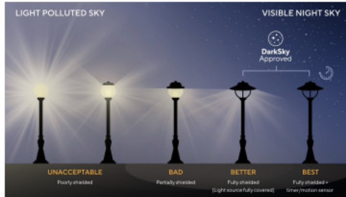
Graphic showing unacceptable vs DarkSky-approved lighting fixtures
